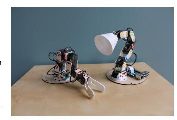
Motors configuration: in order for the motors to be connected and identified on the same line, they must have a unique ID. You will get them all set to the same ID. You should set a new and unique ID to each of the motors.
